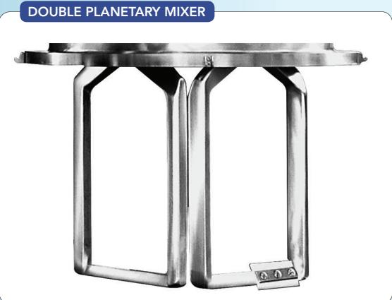
Figure 1. Two rectangular stirrers that rotate on their own axes as they revolve on a common axis move through the batch continuously mixing materials up to about 2 million cP.
