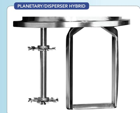
Figure 2. Unit combines a high-speed disperser and a rectangular or helical planetary blade that transports non-flowing, viscous materials from the sidewall to the high-shear device.
