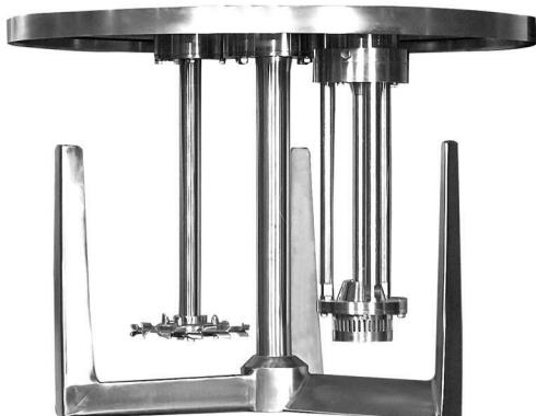
Figure 4. The 3-wing anchor stimulates greater flow in the mix vessel and moves material toward two stationary high-shear agitators, increasing their effective viscosity range.
