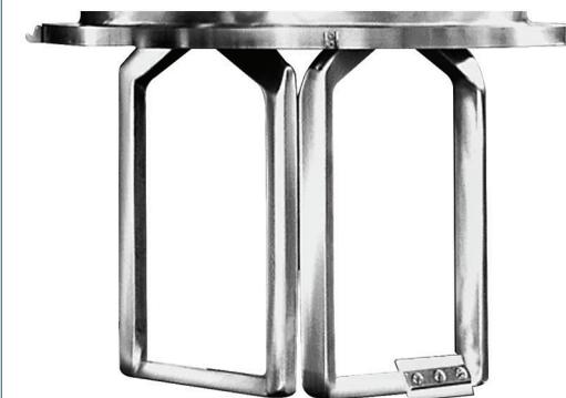
Figure 1. Two rectangular stirrers that rotate on their own axes as they revolve on a common axis move through the batch continuously mixing materials up to about 2 million cP.
