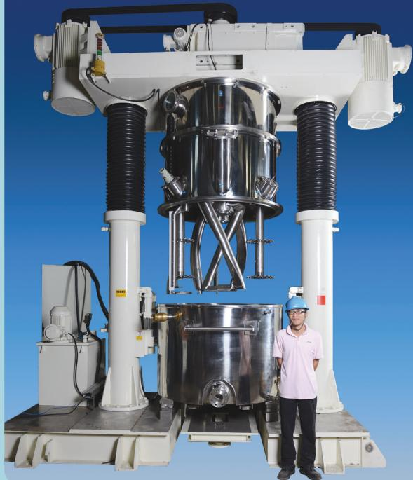
Figure 5. This 300-gallon unit is used for lithium-ion battery production in China; 750-gallon mixers will be online soon and even larger devices are coming.
