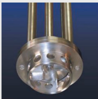
The single-stage rotor/stator high-shear mixer is still used widely today in a multitude of industries, often replacing high-speed dispersers.
