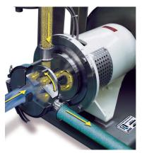
In the SLIM system, a large volume of powder (shown in yellow) is drawn into the high shear zone, where it is simultaneously combined and mixed with the liquid stream (blue). Agglomerates have no opportunity to form. Particles are broken apart and even hard-to-disperse powders are dispersed instantly in the liquid stream.
