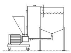
A single SLIM system generally serves multiple mix vessels. Batch material flows from the vessel to the mixer where it is subjected to intense shear. It then flows back into the vessel for recirculation, which continues until the target particle/droplet size distribution has been achieved.
