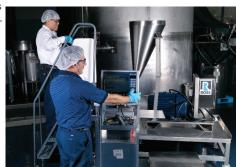
Joe Piazza, VP Operations, is shown initiating the batch process on the SLIM system control panel, while another operator prepares to charge the mixer through the unit's overhead hopper. The ingredients will be drawn into the high shear chamber and dispersed instantly into a stream of liquid drawn from this 2,500gallon vessel.
