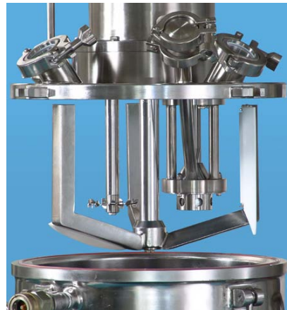
Triple-Shaft Mixer with Three-Wing Anchor Agitator, High Speed Disperser and High Shear Rotor/Stator with SLIM (Solids/Liquid Injection Manifold). The SLIM is utilized for sub-surface addition of powders that tend to dust or form agglomerates.
