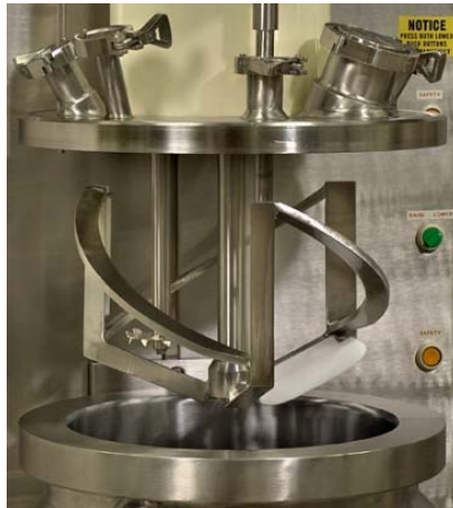
Dual-Shaft Mixer with Three-Wing Anchor Agitator and High Speed Disperser. The Anchor Agitator's dished shape matches the mix vessel's profile.
