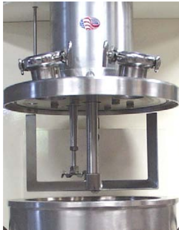
Dual-Shaft Mixer with Two-Wing Anchor Agitator and High Speed Disperser.
