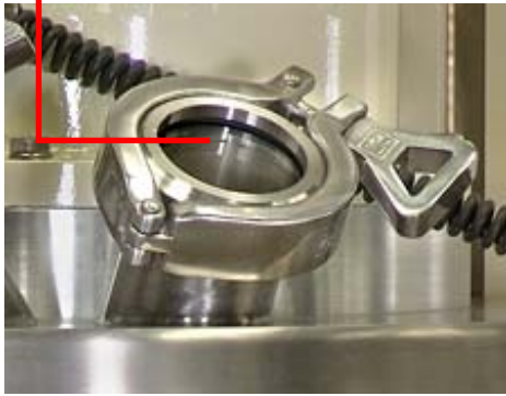
Each sight port includes gaskets and a stainless steel quick-release clamp.
