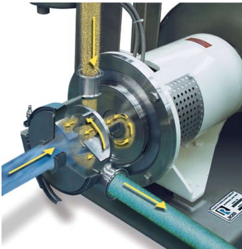
FIGURE 3. This illustration shows how a powder-induction mixer works. The liquid stream (blue) enters the mixer and immediately encounters the powder addition. Drawn by a powerful vacuum, free-flowing powders (yellow) are injected into the liquid and instantaneously mixed under high shear. The resulting dispersion (green) is expelled centrifugally through the stator openings at high velocity
