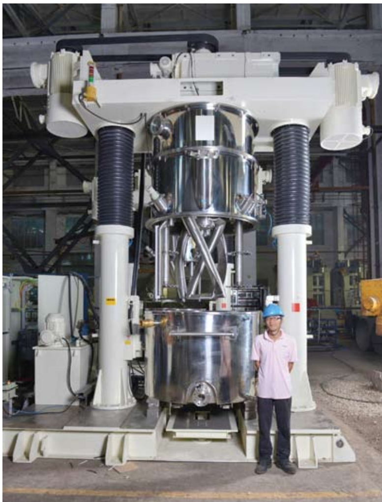
FIGURE 2. The agitators in this 300-gal planetary disperser are lifted out of the vessel via a dual-post hydraulic lift, allowing complete access for cleaning and maintenance
