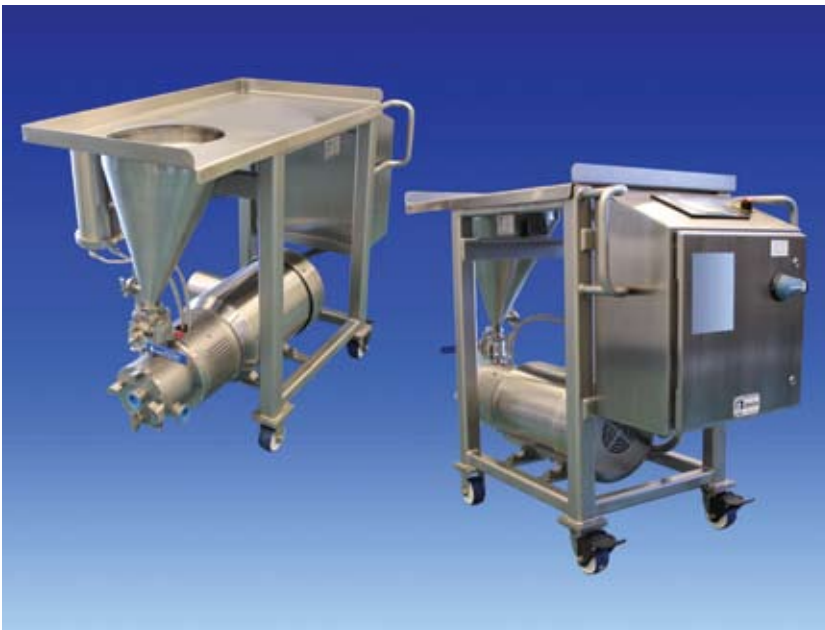
FIGURE 4 (above). Combining this powder-induction mixer with a work bench eases material handling. This mobile system pumps liquid from a tank, while simultaneously drawing powders from a built-in hopper. The resulting mixture is pumped by the mixer back into the tank and recirculated until dispersion is complete
