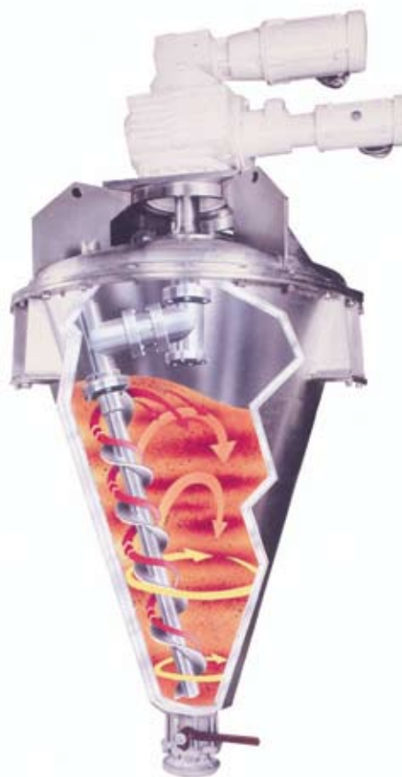
FIGURE 6. The agitator movement and material flow pattern shown here for a vertical blender-dryer provides favorable results for many applications. Product is heated through contact with the jacketed sidewalls. The vacuum-rated cover may also be jacketed to avoid condensation
