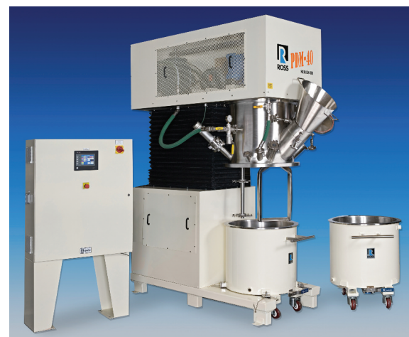
A hybrid planetary mixer featuring a rectangular stirrer blade and disperser shaft with two disc blades. The change-can feature allows for semi-continuous processing.
