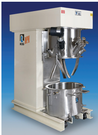
Double Planetary Mixer with patented High Viscosity "HV" blades capable of mixing extremely viscous products as high as 8million cps. The mixer in this photo is a "reverse lift" design wherein the mix can is raised up and down, instead of the stirrers. The stationary ports can be hard-piped to accept mix ingredients.
