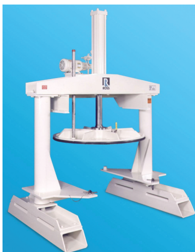
Floor-mounted platen-style hydraulic discharge system. Viscous product is forced out through a valve in the side or bottom of the vessel, or through the top of the platen. A discharge system eliminates wasted hours of scraping heavy or sticky materials from a mix vessel.
