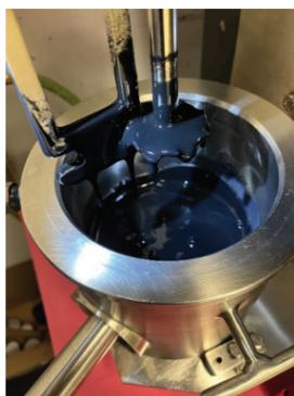
FIGURE 2. The Ross PowerMix 0.5-gal capacity mixer produces homogeneous slurries for battery electrode development
