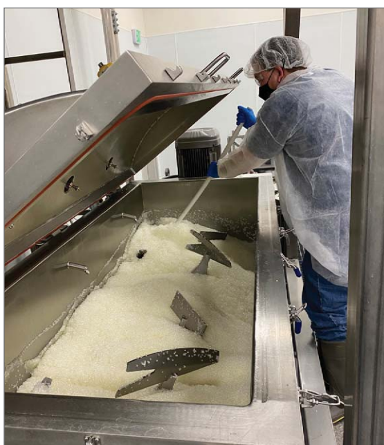
IBF's scented beads undergo a unique and complex manufacturing process that requires appropriately timed oil inclusion and continuous deep vacuum in the Ross 36-cu-ft paddle blender.
