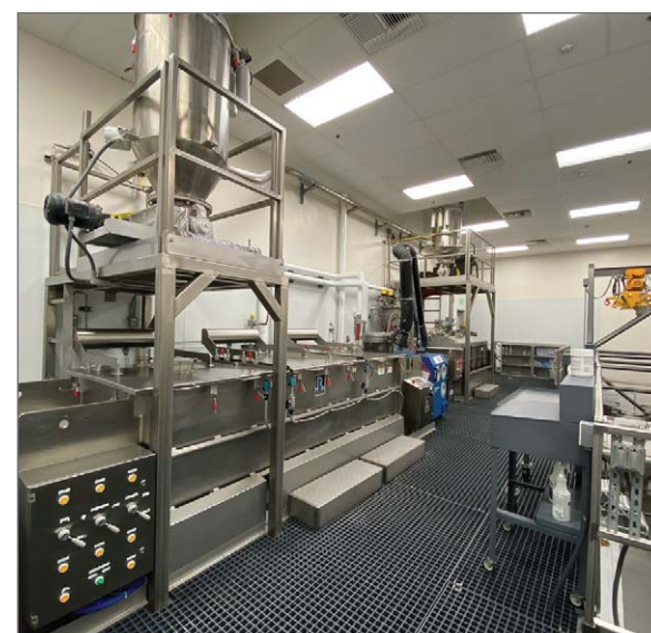
IBF currently has seven Ross paddle blenders in various sizes in configurations currently used to manufacture air fresheners, bath salts, laundry enhancers, and a range of other products.
