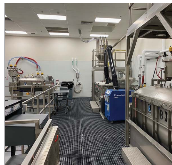
Made from US steel, the Ross 10-cu-ft paddle blender features precisely designed paddle agitators, a 10-gal liquid fragrance delivery spraying system, and multiple automated valves operated from a main touchscreen control panel.
