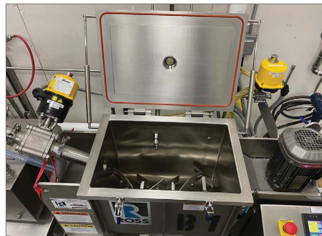
This portable Ross 1-cu-ft paddle blender is used for R&D testing and making pilot scale batches.
