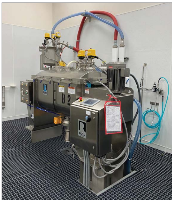
Made from US steel, the Ross 10-cu-ft paddle blender features precisely designed paddle agitators, a 10-gal liquid fragrance delivery spraying system, and multiple automated valves operated from a main touchscreen control panel.
