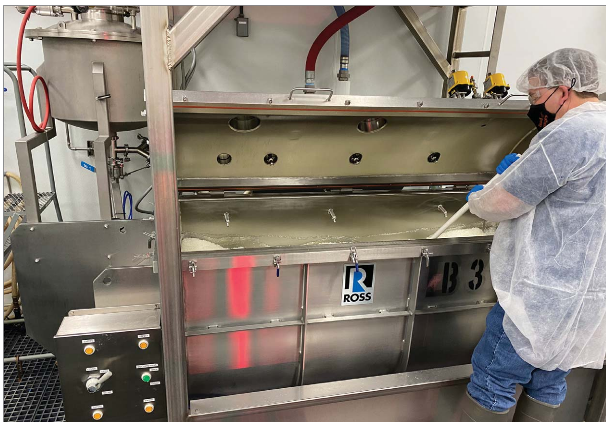
Made from US steel, the Ross 10-cu-ft paddle blender features precisely designed paddle agitators, a 10-gal liquid fragrance delivery spraying system, and multiple automated valves operated from a main touchscreen control panel.
