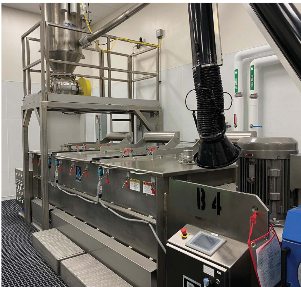
This atmospheric design Ross 100-cu-ft paddle blender is equipped with a pneumatically-actuated three-piece cover with custom ports, as well as spray nozzles for cold and hot water supply.
