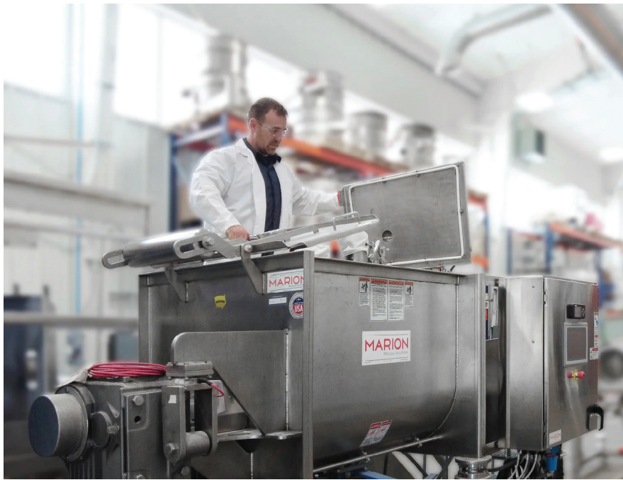
Mixers and blenders should also offer access and easy viewing of surfaces for cleaning and inspection personnel.
