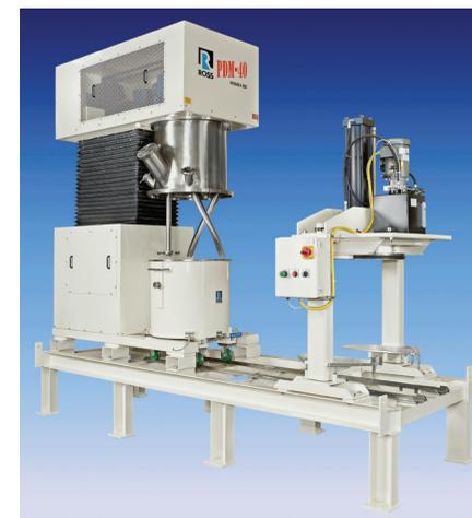
*Figure 3. A hybrid planetary mixer equipped with a high-speed disperser and helical planetary stirrer. After mixing, the vessel is rolled over to the discharge station. A platen is lowered hydraulically into the vessel, forcing product out and into pails positioned under the raised platform.*
