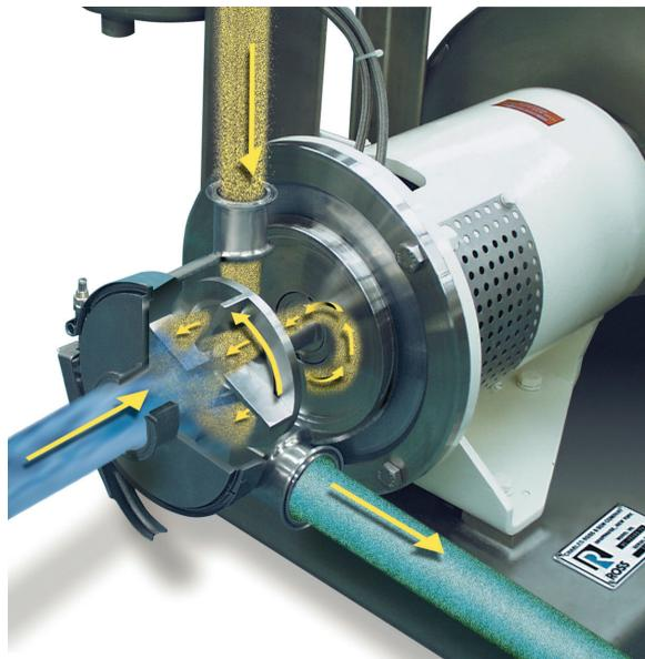
*Figure 1. How a powder induction mixer works: the liquid stream (blue) enters the mixer and immediately encounters the powder addition. Drawn by a powerful vacuum, free-flowing powders (yellow) are injected into the liquid and instantaneously mixed under high shear. The resulting dispersion (green) is expelled centrifugally through the stator openings at high velocity.*
