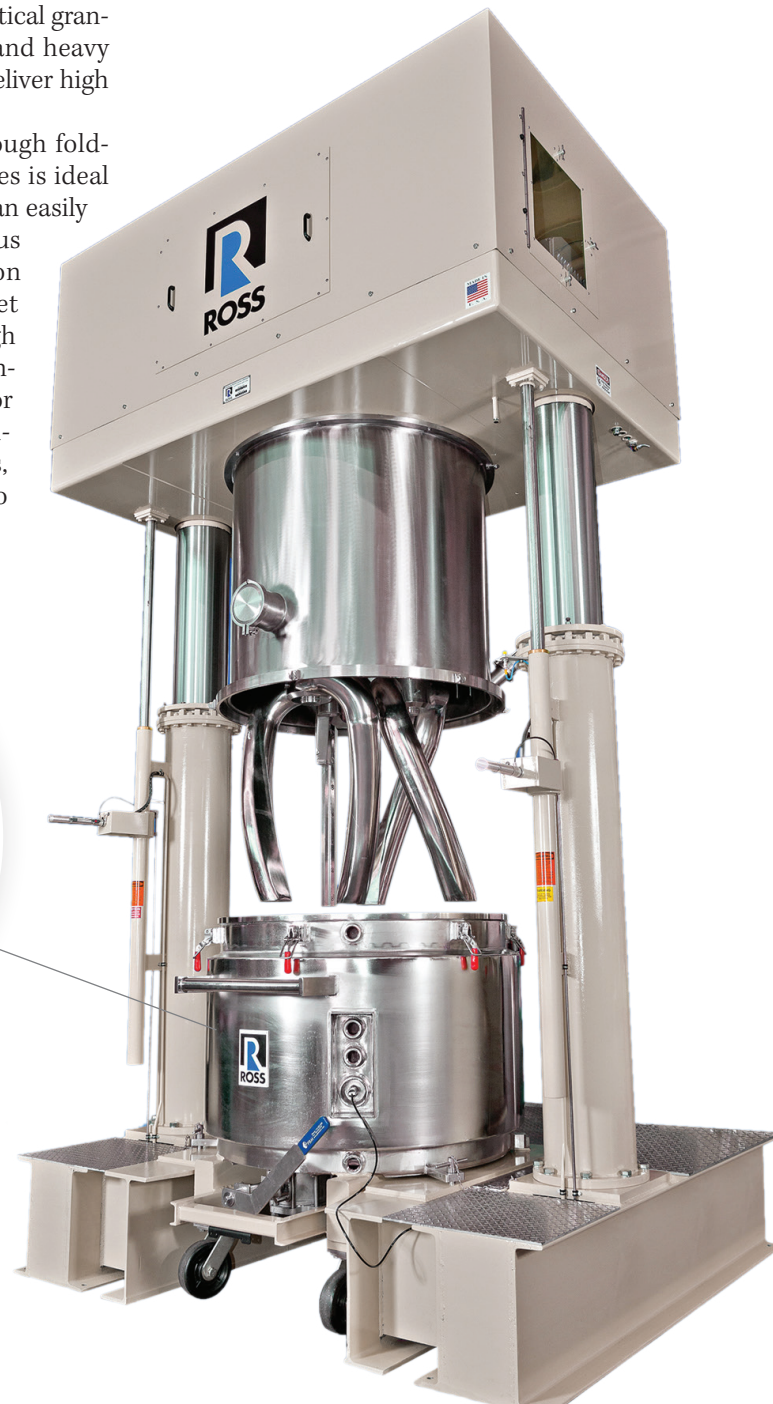
↑ Figure 1. Double planetary mixer with helical high-viscosity (“HV”) blades designed for materials up to around 6 million centipoise (U.S. Patent No. 6,652,137).
