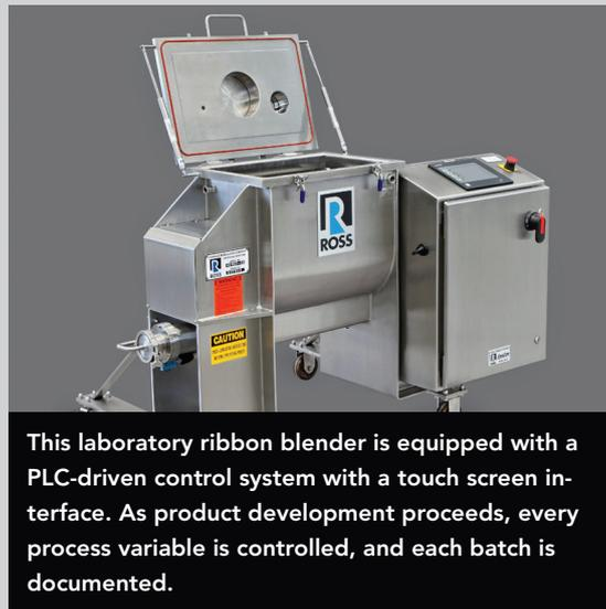
This laboratory ribbon blender is equipped with a PLC-driven control system with a touch screen interface. As product development proceeds, every process variable is controlled, and each batch is documented.
