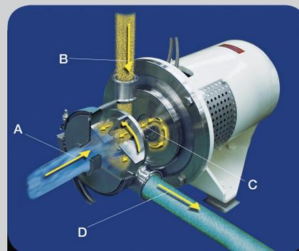
In the SLIM (Solid/Liquid Injection Manifold) powder-injection system, a liquid stream (A) enters the high-speed rotor. Drawn into the mixer by a powerful vacuum, the powder (B) is injected through the ported rotor (C) directly into the high-shear zone, where it is subjected to intense shear. With particles instantly dispersed, the resulting product is ejected from the mixer (D).
