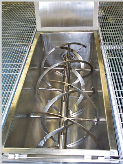
A ribbon blender engineered for sanitary applications includes high-grade stainless steel construction, a sanitary finish, close tolerances, and design details that eliminate corners and crevices where batch material might collect.
