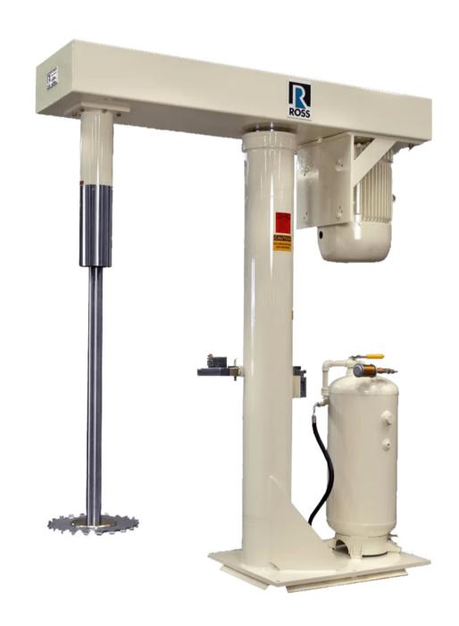
The ROSS floor-mounted Model HSD-50 high-speed disperser with explosion-proof 50HP motor, heavy-duty V-belt drive and bearings, an air/oil hydraulic lift, and a high-quality, laser cut, 16-inch diameter blade.
