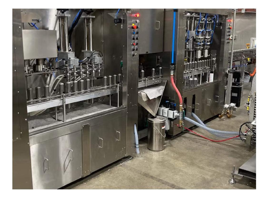
To keep up with growing demand, Chem-Pak recently installed a new high-speed aerosol production line to accommodate thicker compounds.
