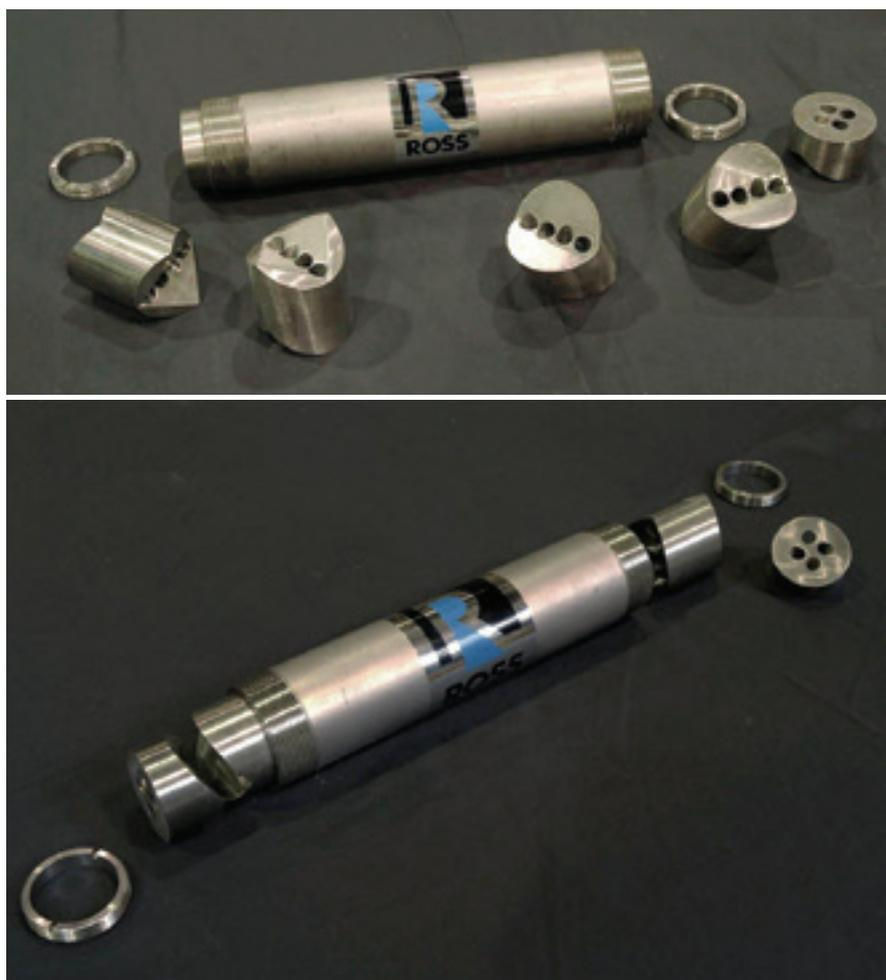
Interfacial surface generator (U.S. patent number US3404869), a static mixer designed for high-viscosity, laminar-flow applications.
