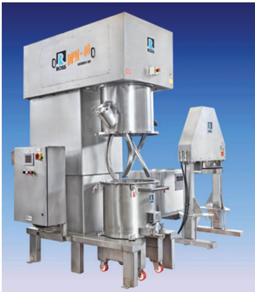
Double-planetary mixer with discharge system, in all-stainless steel construction, designed for production of hydrogel adhesives used in sterile wound dressings. The helical blades handle ultra-high viscosities up to around 6 million cP.
