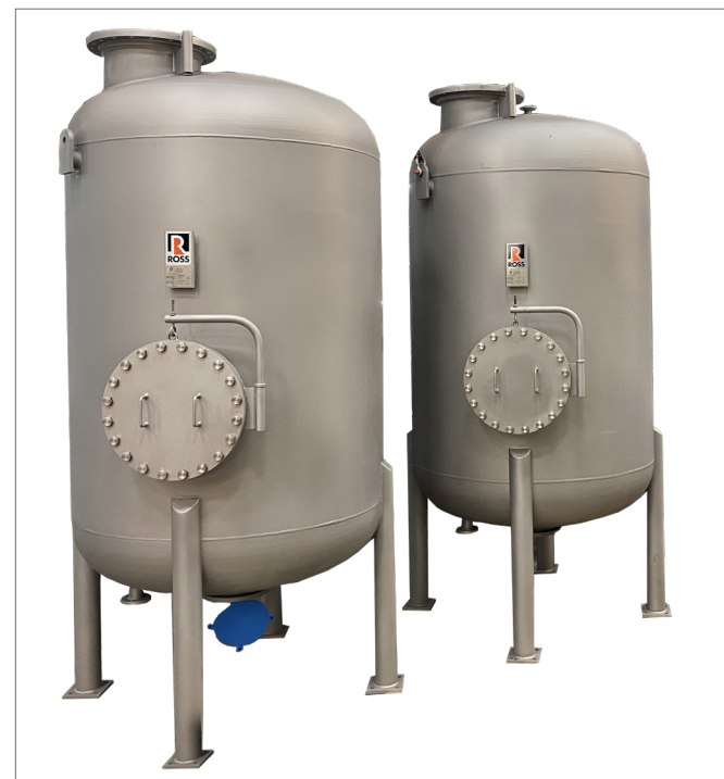
This ROSS 3,000-gal 304/304L stainless steel-type elevated tanks with dished bottom are ASME stamped and designed for 200 psi with full vacuum up to 200°F.
