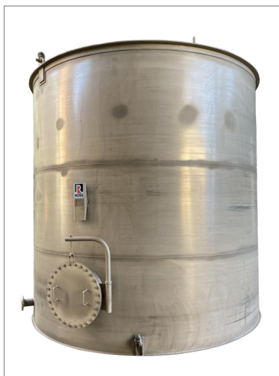
This ROSS 4,500-gal 304/304L stainless steel-type flat-bottomed tank is ASME stamped and designed for 25 psi with full vacuum up to 400 °F.
