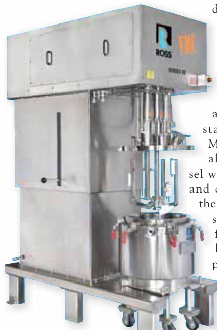
Dual-shaft mixer with three-wing anchor and multiple saw-tooth disperser blades.
