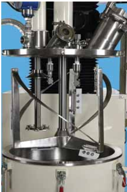
Agitation system of a multi-shaft mixer featuring a three-wing anchor with helical flights and Teflon scrapers, as well as a saw-tooth disperser with slinger to prevent batch material from climbing up the high-speed shaft.
