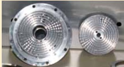
to 11,300 fpm). This combination subjects the product to intense shear in every pass through the rotor/stator. The gap between adjacent surfaces of the rotor and stator are adjustable from 0.010-0.180 in. for fine-tuning shear levels and flow rates.
