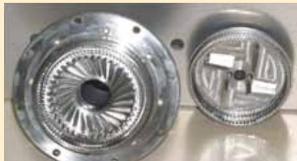
pumping vanes. Different streams are induced within the grooves and collide at high frequency before exiting the mix chamber.
