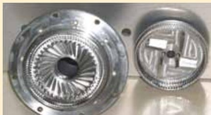
The MegaShear head (U.S. patent number 6,241,472) operates at the same tip speed as the X-Series and QuadSlot heads, but it is more aggressive in terms of shear and throughput levels. It consists of parallel semi-cylindrical grooves in the rotor and stator, toward which product is forced by high-velocity pumping vanes. Different streams are induced within the grooves and collide at high frequency before exiting the mix chamber.
