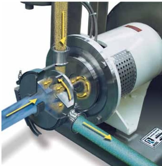
Figure 1. The ported rotor generates an intense vacuum that draws hard-to-disperse powders such as fumed nanosilica into the mix chamber. The powders are injected directly into the high shear zone and dispersed into the liquid stream.
