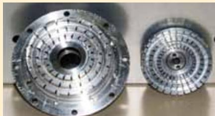
The X-Series head (U.S. patent number 5,632,596) consists of concentric rows of intermeshing teeth. The product enters at the center of the stator and moves outward through radial channels in the rotor/stator teeth. Tolerances are extremely close and the rotor runs at very high tip speeds (typically up
