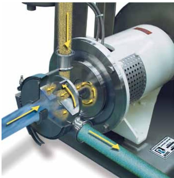
Figure 1. The ported rotor generates an intense vacuum that draws hard-to-disperse powders such as fumed nanosilica into the mix chamber. The powders are injected directly into the high shear zone and dispersed into the liquid stream.
