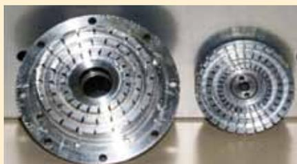
The QuadSlot mixing head is a multi-stage rotor/stator with a fixed clearance. It is used for applications where very high shear levels are required. The QuadSlot generator produces higher pumping rates and requires higher horsepower than a similar size X-Series rotor/stator set.
