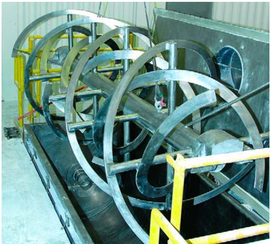
A flat-flange, clamshell coupling allows operators to raise the ribbon agitator out of the blender without moving the end shafts, bearings, or seals, saving hours of time between batches.
