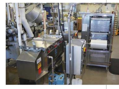
To ensure the homogeneity of various soup products in final packaging, the Heinz team pumps finished soup to a Ross ribbon blender, where continuous agitation prevents garnishes from settling. The product enters the blender through the cover and is pumped from a discharge valve beneath the blender directly to filling equipment alongside the blender. Source: Charles Ross & Son Company.
