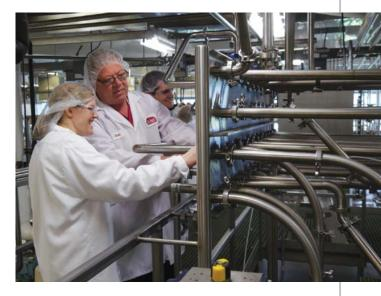
Process equipment and feed lines in the plant are interconnected through hard-piped "process zones." Working like giant switchboards, these manifolds simplify changeover, increase production and make the plant more responsive to customer needs. Source: Charles Ross & Son Company.
