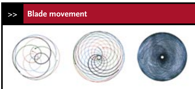
Figure 3. In a double planetary mixer, the orbital motion of blades is both predictable and efficient.
