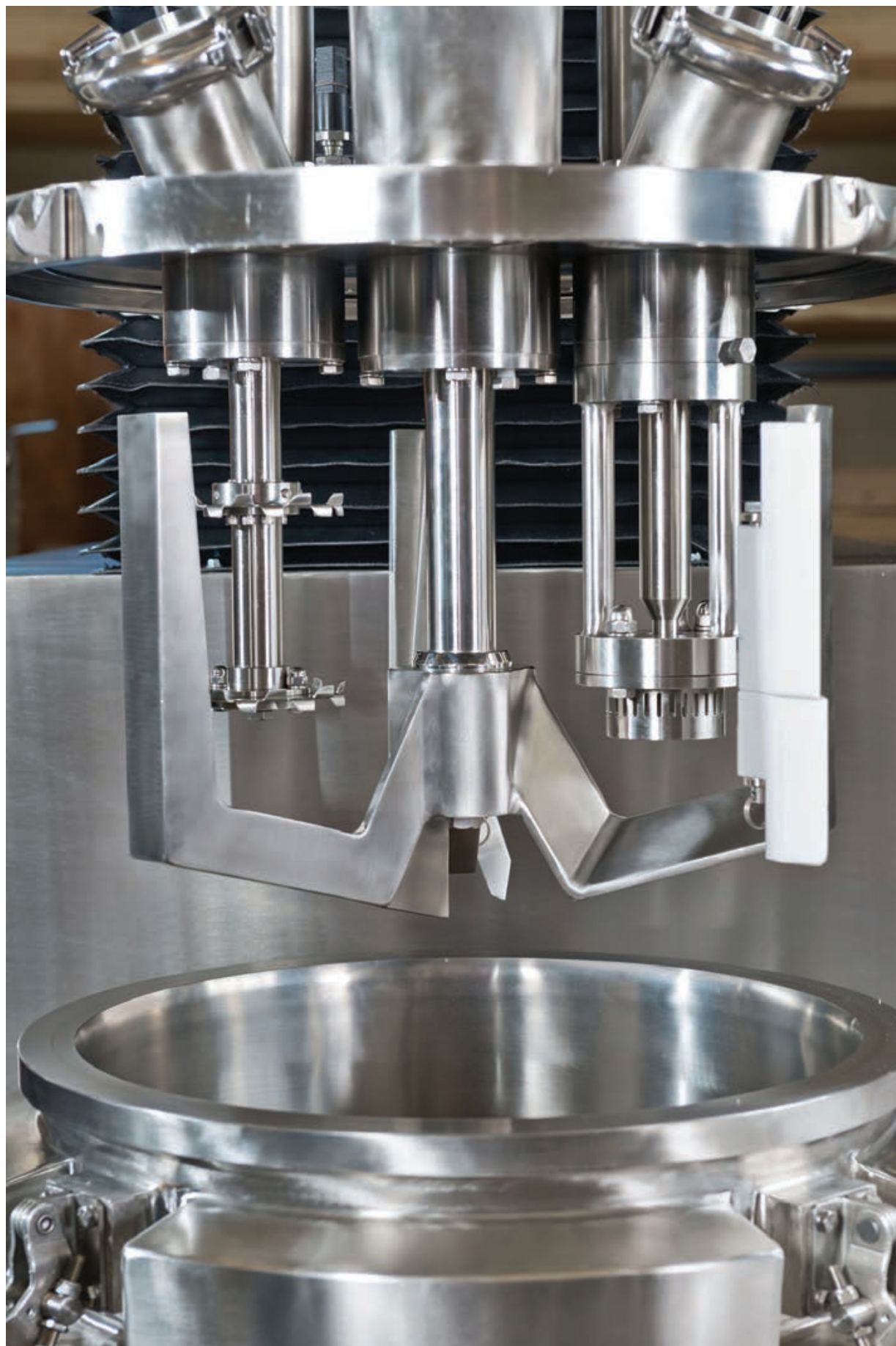
→ Figure 1: Multi-shaft mixer designed for single-pot processing of viscous and air-free gel formulations. All images courtesy of Charles Ross & Son Company
