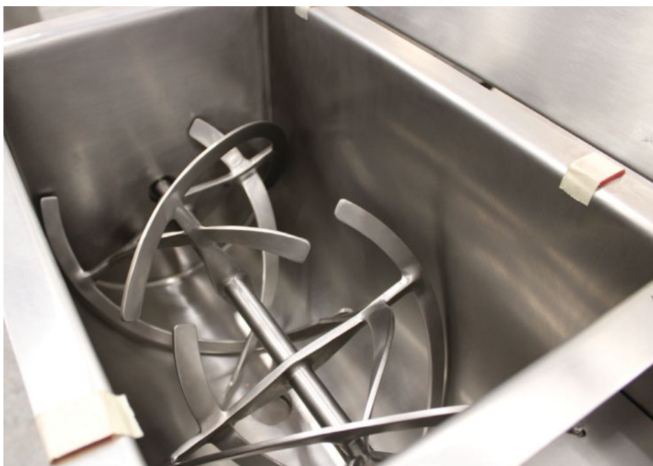
▲ A ribbon blender's outer ribbons direct material inward towards the center of the trough, while the inner ribbons move material outward, creating radial flow as well as two-way axial flow.
