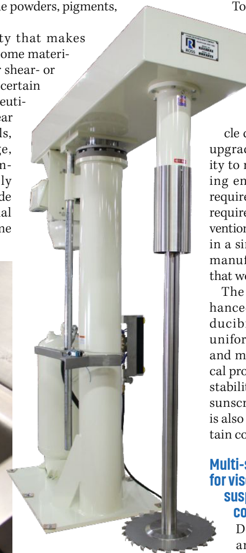
▲ High-speed dispersers feature open-disc blades that run with a tip speed of roughly 5,000 fpm, generating a vortex for rapid, even incorporation of dry ingredients.
