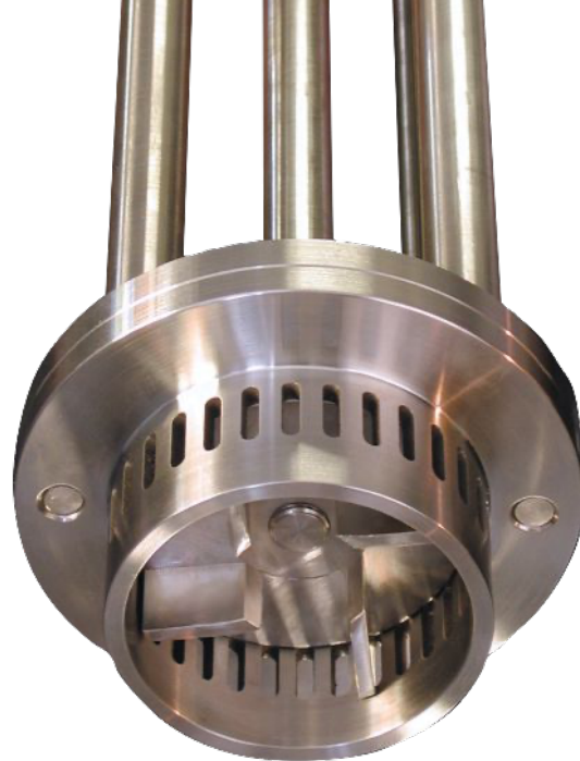
▲ High-shear mixers use a single-stage, four-blade rotor that spins at high speed within a stationary stator. As the blades pass the stator openings, they expose particles to high shear forces, expelling material into the surrounding mix while the spinning rotor draws more material into the mixer head.
