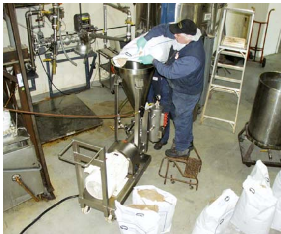
The SLIM in-line rotor/stator powder injection system from Charles Ross & Son can be wheeled between TFF’s several 1,000-gallon vessels as well as the open-head tank. Source: Charles Ross & Son.
