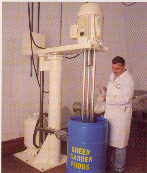
A Ross single-stage, 30 hp batch unit with a 7-inch diameter rotor and an electronic variable speed control allows Green Garden Foods to adjust shear rates and throughput.
