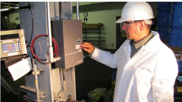
Using a Variable Frequency Drive, the operator slows the mixer to continue recirculation under lower shear conditions.
