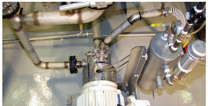
The inline SLIM Solid/Liquid Injection Manifold instantly disperses powders in a liquid stream. A specially designed rotor/stator generator develops an intense vacuum, which draws the powder through the powder injection inlet to the high shear zone, where it is dispersed instantly. An auxiliary pump and eductor are not required.
