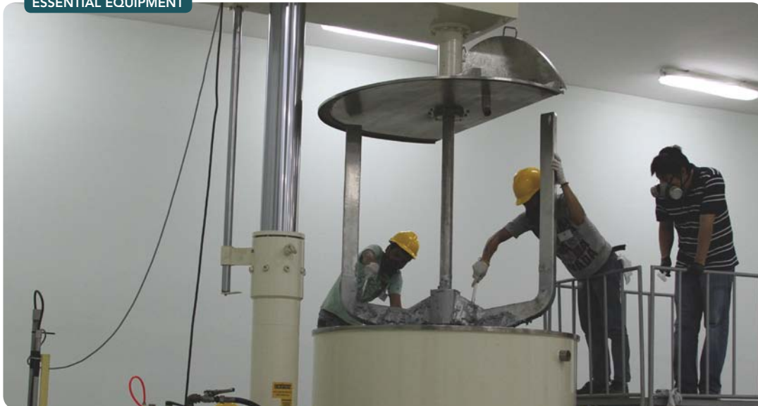
Figure 2. This high-capacity mixer, manufactured in one of Ross's plants in China and shown being installed in new plant in Jakarta, Indonesia, plays a crucial role in production of high-performance coating.
