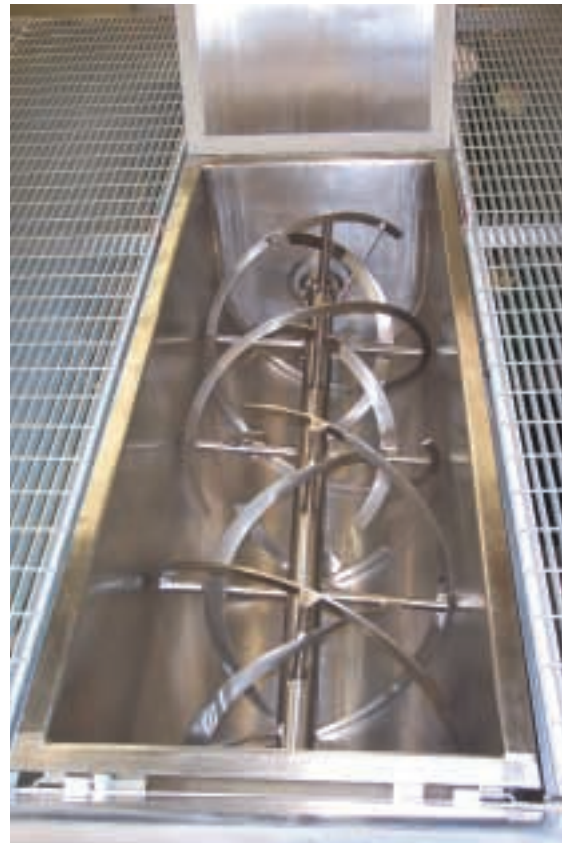
Raw materials are charged on the overhead mezzanine. A balanced ribbon design provides vigorous lateral and axial movement of the bulk material, then promotes fast center discharge.
