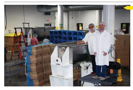
quire extended blending times for color development. "Since the installation of the 42N-25, the required blending time for these blends has been reduced by a third. We have also noticed an increase
