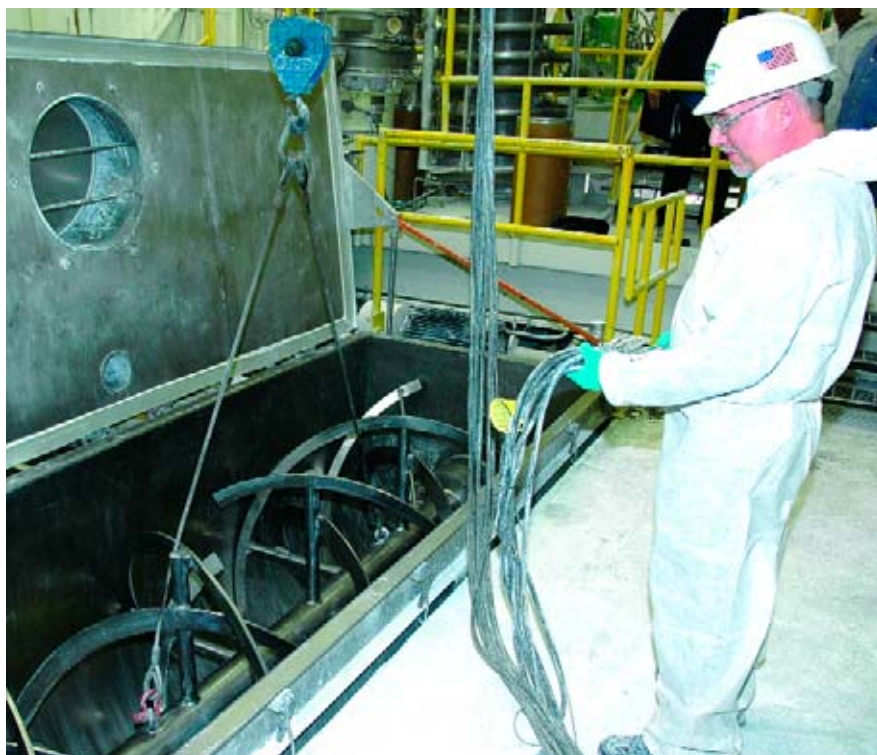
The removable ribbon is hoisted out using an overhead crane so operators can quickly and easily clean both the ribbon and the blender's trough.
