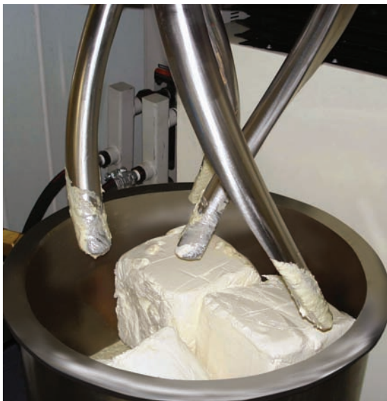
The trailing slope and helical design of the Ross mixer blade works well in this specialty cheese application, creating five times the product in half the time of a conventional mixer. Source: Charles Ross & Son.
